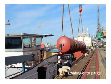
Multimodal transportation included road transportation to point of loading, where the route was agreed and confirmed with local road authorities; civil works on route were done using a 3D Scan for the most difficult parts of the route.
