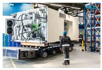
A self propelled modular trailer (SPMT) was used to move the press measuring 6.90 metres long, 3.90 metres wide and 3.10 metres high into the factory.
